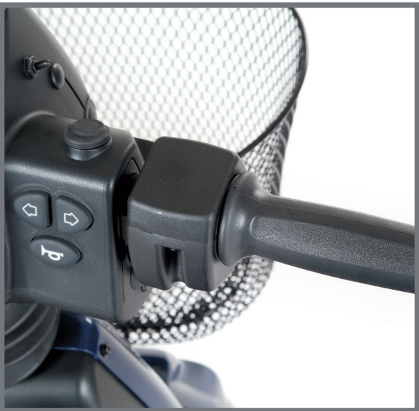
Twistgrip throttle control left and right
