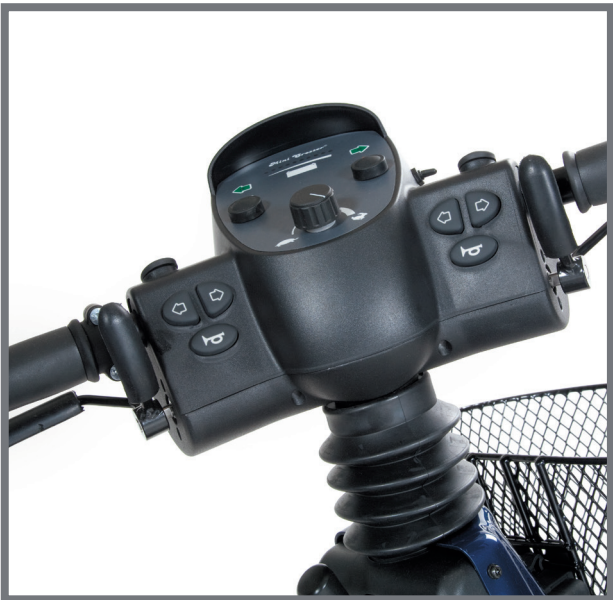
Left and right accelerator, with switch
